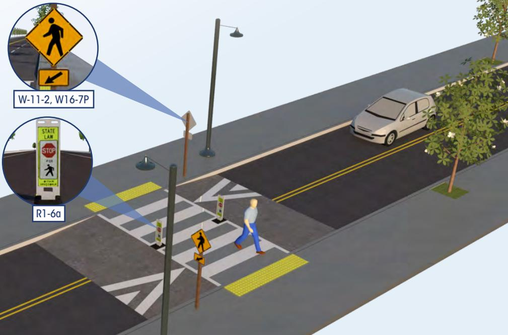
Raised crosswalks are ramped speed tables spanning the entire width of the roadway, often placed at midblock crossing locations. The crosswalk is demarcated with paint and/or special paving materials. These crosswalks act as traffic-calming measures that allow the pedestrian to cross at grade with the sidewalk.
