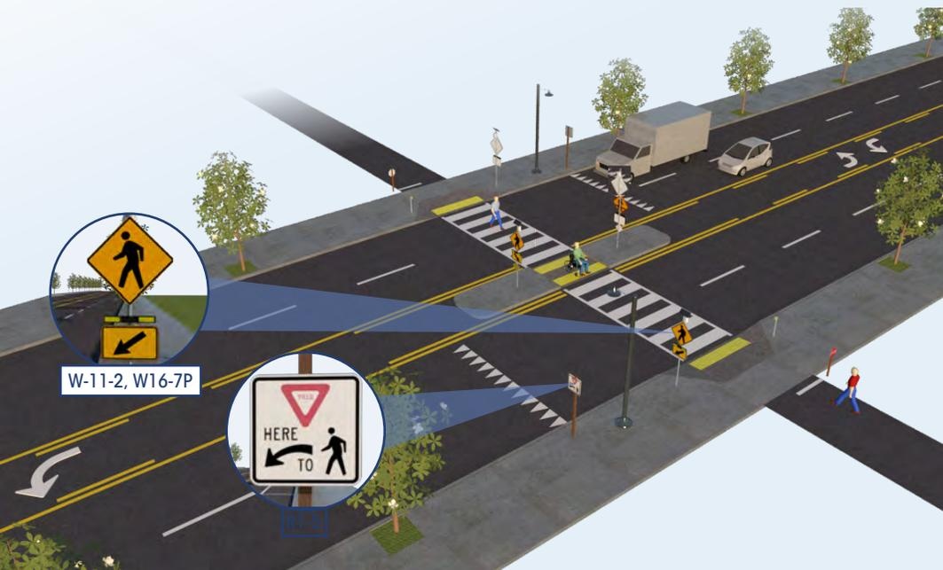
RRFBs are pedestrian-actuated conspicuity enhancements used in combination with a pedestrian, school, or trail crossing warning sign to improve safety at uncontrolled, marked crosswalks. The device includes two rectangular-shaped yellow indications, each with an LED-array-based light source, that flash with high frequency when activated.
