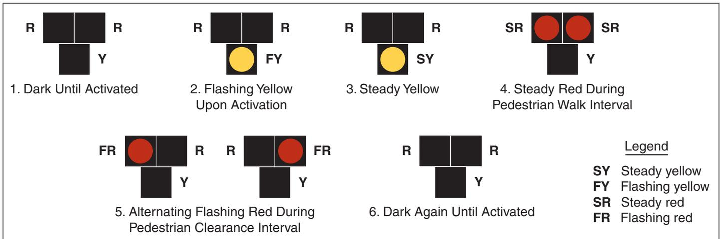
When a pedestrian activates a PHB, a flashing yellow light is followed by a solid yellow light, alerting drivers to slow. A solid red light requires drivers to stop while pedestrians have the right-of-way to cross the street. When the pedestrian signals display a flashing DON'T WALK indication, the overhead beacon flashes red, and drivers may proceed if the crosswalk is clear.
