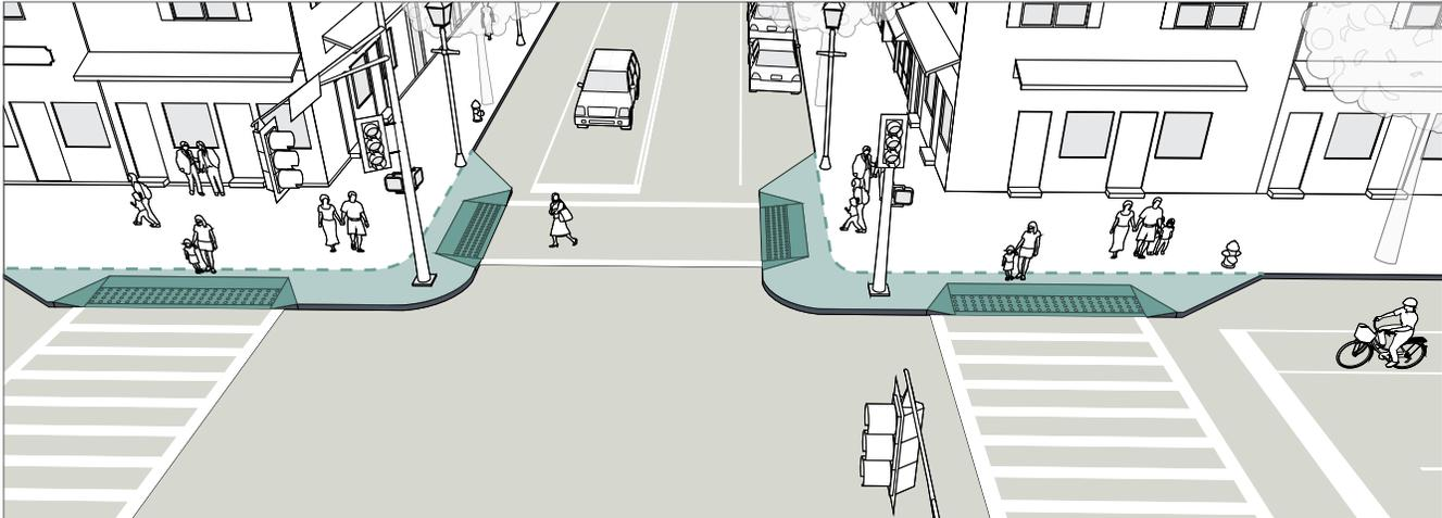
A **Curb Extension** or “**Bulb Out**” extends the sidewalk or curb line into the street or parking lane, thus reducing the street width and improving sight distance between the driver and pedestrian. A curb extension is a candidate treatment for any uncontrolled pedestrian crossing, particularly where parking lanes exist. Curb extensions should not extend into paths of travel for bicyclists. See Appendix C for separate technical sheet and Figure 3.
