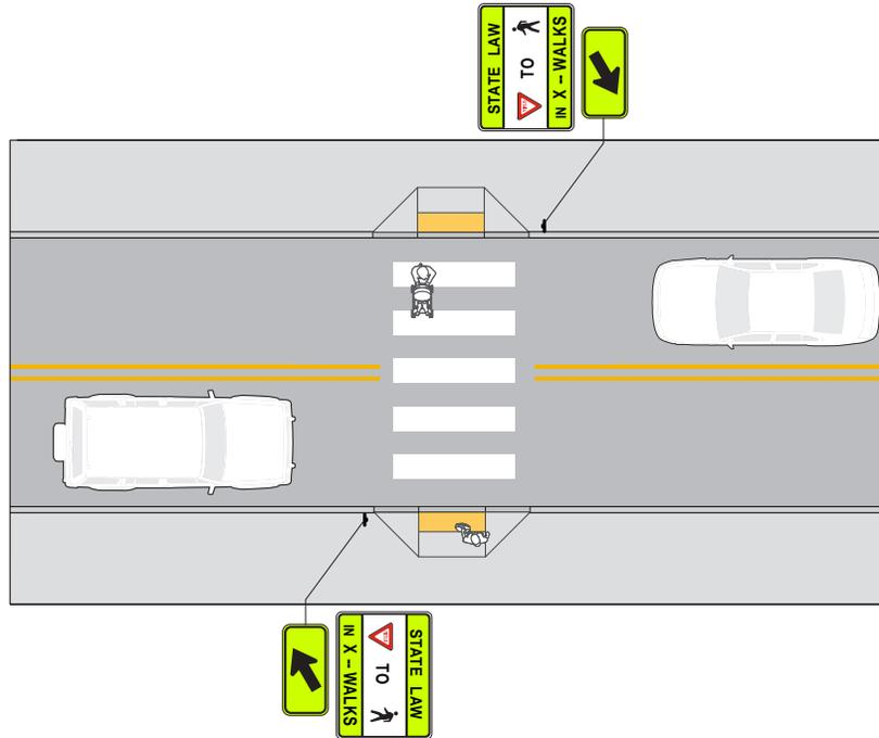
**C1** Figure 11: High visibility markings, “state law” signage (modified R1-6), side/median mounted yield signs, and advanced yield lines
