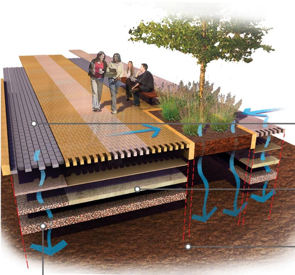
Spaces between the *permeable pavers* direct water to a series of layers below the pavement sub base.
