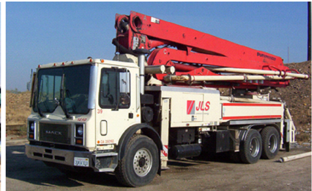
Figure 10 Concrete Pump Truck
