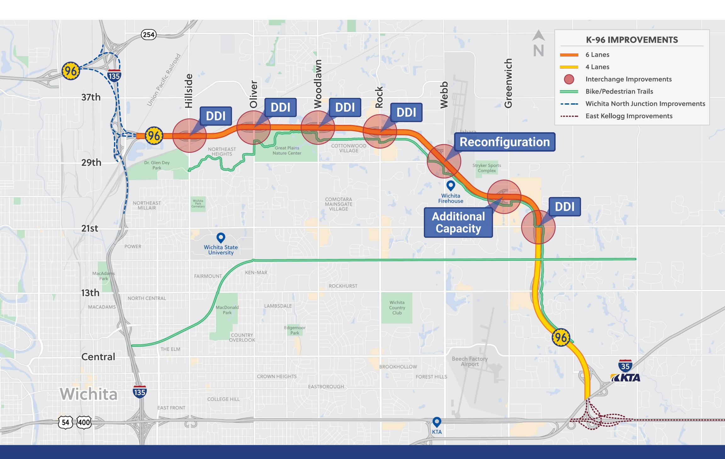
The K-96 Improvements Project extends from the K-96 and I-135 interchange (near Hydraulic Avenue) approximately 9.5 miles east/southeast to north of the K-96/U.S. 54/400 interchange. The project will explore pavement replacement, adding new lanes and will include improvements to the Hillside, Oliver, Woodlawn, Rock, Webb, Greenwich, and 21st Street interchanges.
