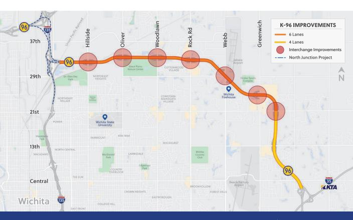
The K-96 Improvements Project extends from the K-96 and I-135 interchange (near Hydraulic Street) approximately 9.5 miles east/southeast to north of the K-96/US 54/400 interchange. The project will explore pavement replacement, adding new lanes and will include improvements to the Hillside, Oliver, Woodlawn, Rock, Webb, Greenwich, and 21st interchanges.
