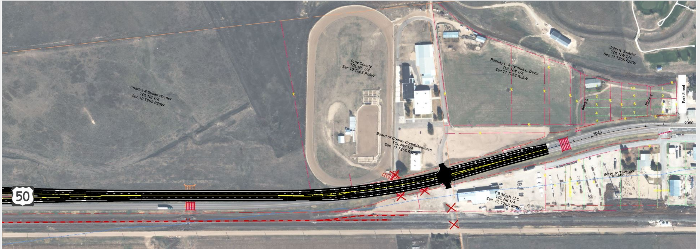
US-50 Expressway Variable Width Median Transitioning to Undivided Section; Fairgrounds Entrance with Turn Lanes at Cimarron
