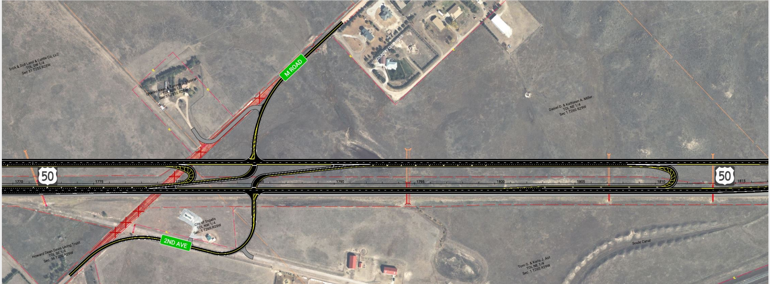
US-50 Expressway with 150' Median; RCUT Intersection at 2 nd Ave./M Road at Ingalls
