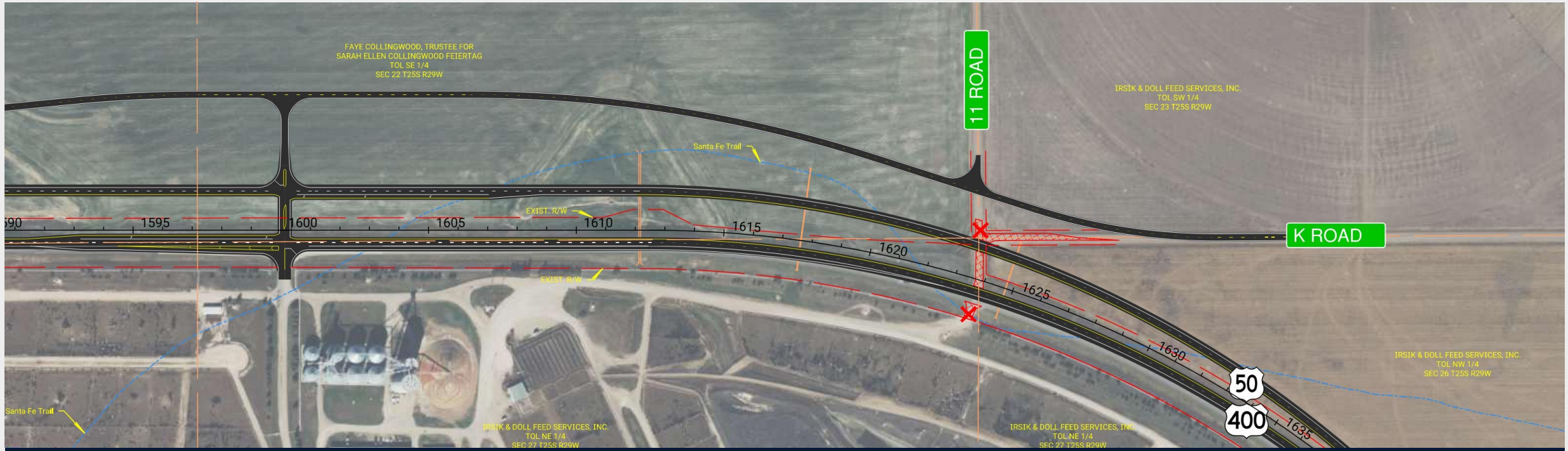
US-50 Expressway with 150' Median; Intersection at 11 Road and Irsik & Doll Feed Lot Entrance
