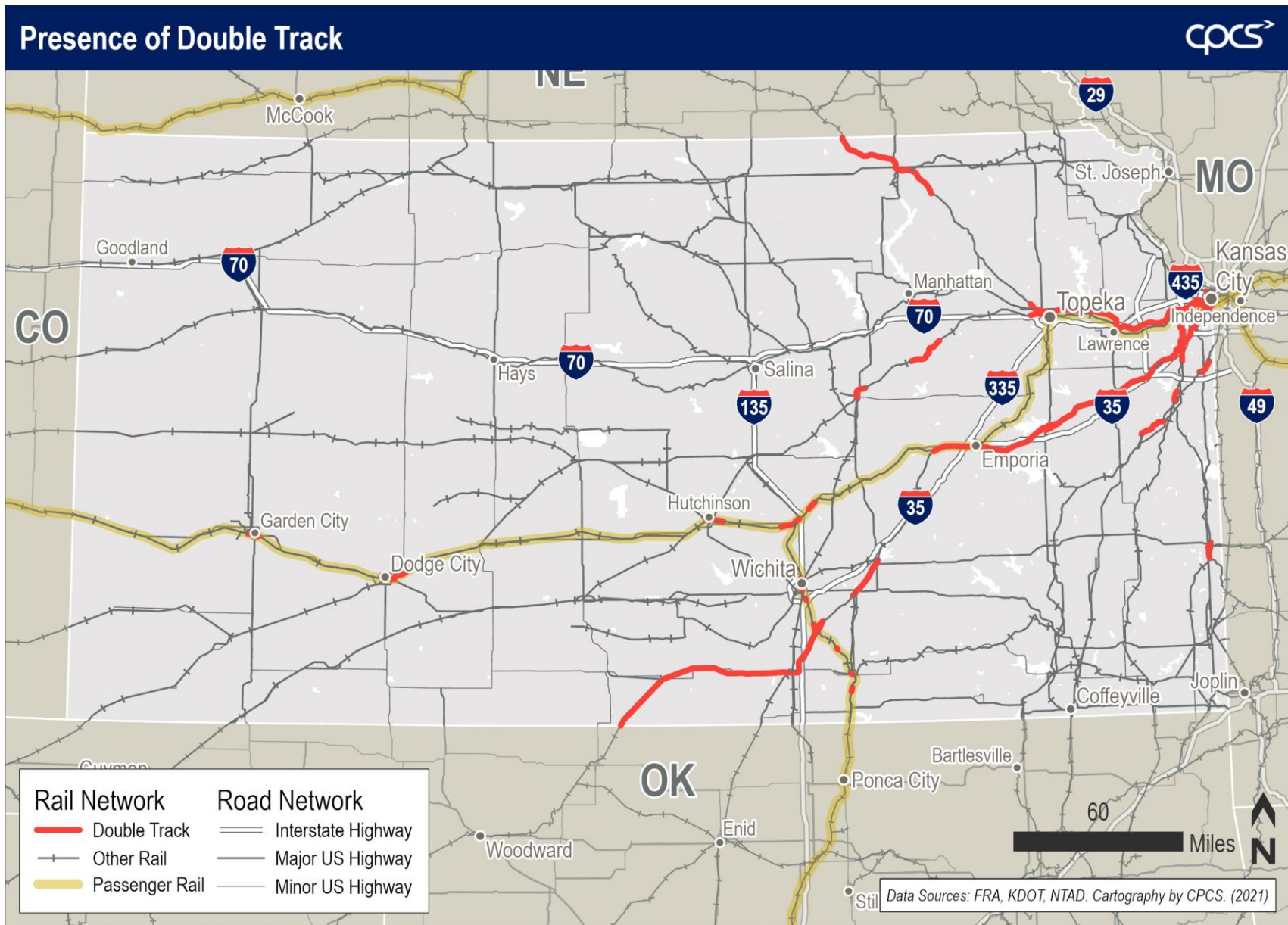
Figure 7-10: Presence of Double Track
