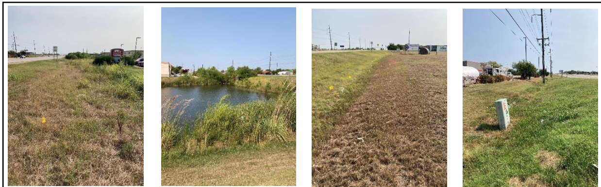
Figure 6.1. Four images showing embankment, ditch, pond, power line poles (bottom right) and buried utilities (indicated with yellow and orange pin flags, top and bottom left).
