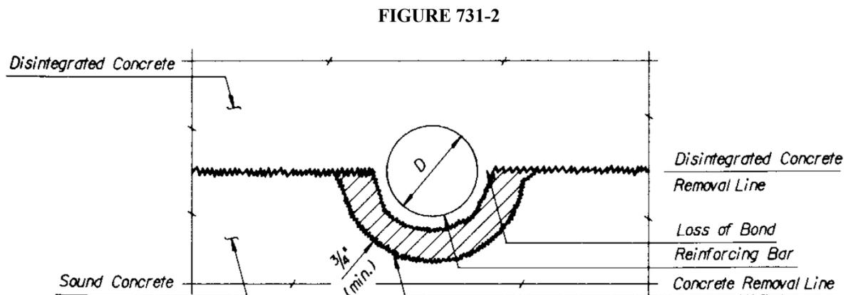
(b) All Reinforcing Bars Other Than the Top Layer of Transverse Bars. Where more than  $\frac{1}{2}$  the diameter of the steel is exposed (**FIGURE 731-3**), or where the bond between existing concrete and reinforcing steel has been destroyed (**FIGURE 731-2**), remove the concrete adjacent to the bars to a depth that shall permit concrete to bond to the entire periphery of the bar with a minimum clearance of  $\frac{3}{4}$  inch.
