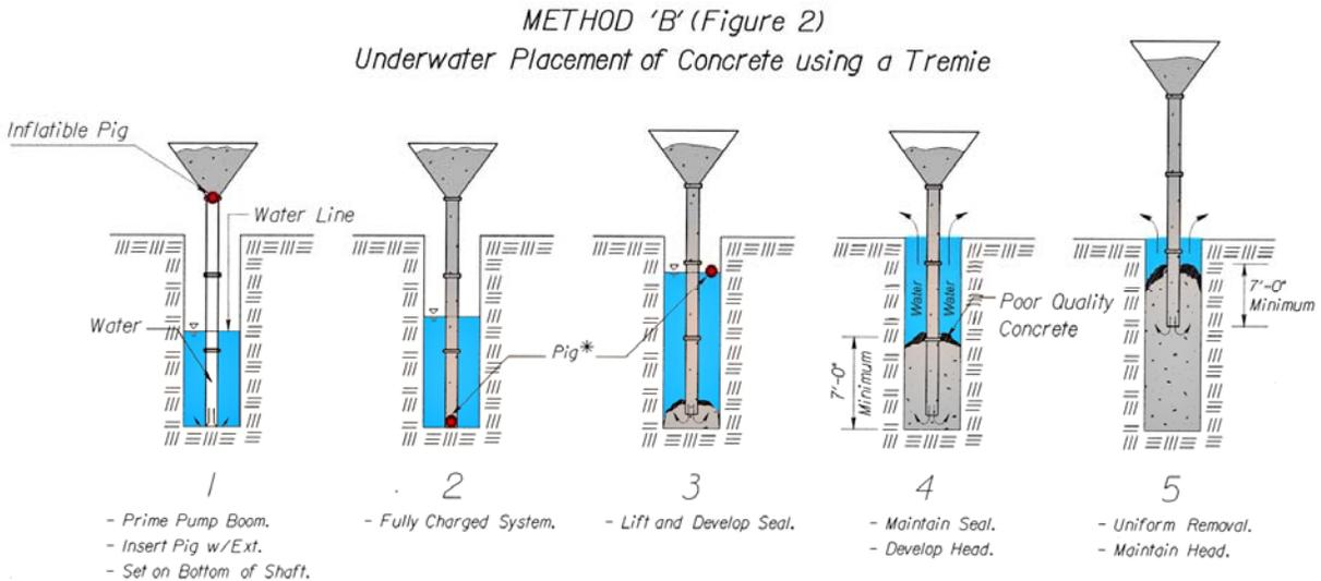
**Method B (Figure 2):** Use a tremie tube, with a pig separating the ground water and concrete, to place concrete into the shaft. Once the tremie tube is resting on the bottom of the shaft, install the pig just below
