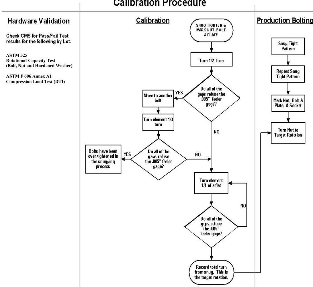
**Installation.** To achieve uniform results, install bolts after performing calibration tightening procedures.
