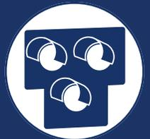
A Pedestrian Hybrid Beacon head consists of two red lenses above a single yellow lens. Unlike a traffic signal, the PHB rests in dark until a pedestrian activates it via pushbutton or other form of detection. When activated, the beacon displays a sequence of flashing and solid lights that indicate the pedestrian walk interval and when it is safe for drivers to proceed (see figure on back page).
