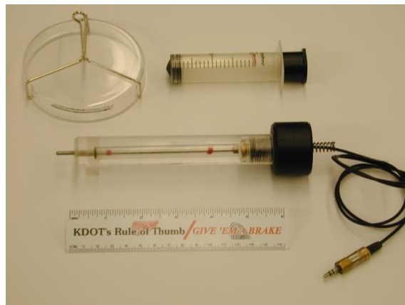
Figure 3 Petri dish, 20 ml syringe, and temperature sensor
